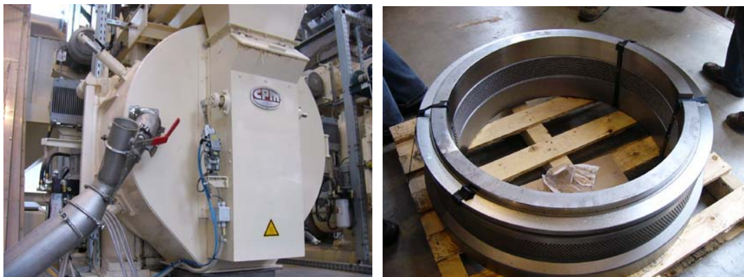
Abb. 1: links: Pelletpresse; rechts: Scheibenmatrize
